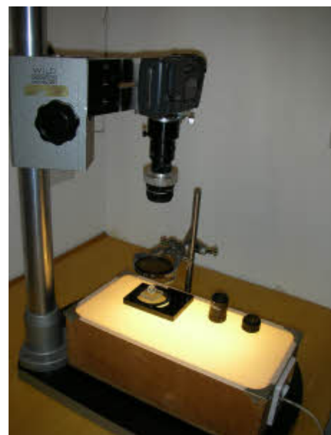
Figure 3. Camera with eyepiece and macro lens being used for transmitted light photography with polarizers.
