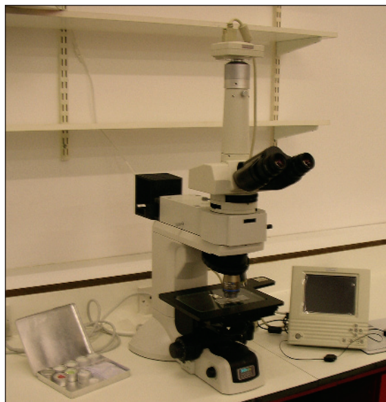
Figure 2: Left: Nikon LV150 metallurgical microscope equipped with an intermediate attachment containing an integral Bertrand lens and a DS 5M L1 camera system.
