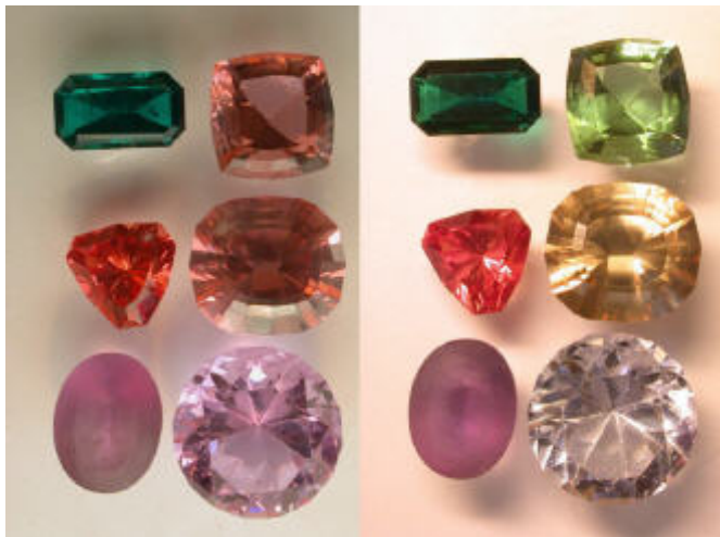
Figure 4.1. Six gems illuminated with tungsten halogen light (left) and fluorescent tube light (right). The gems are (clockwise from top left) hydrothermal emerald, 'tourmalike' glass, coloured cubic zirconia, neodymium glass, amethyst preform and red CZ
