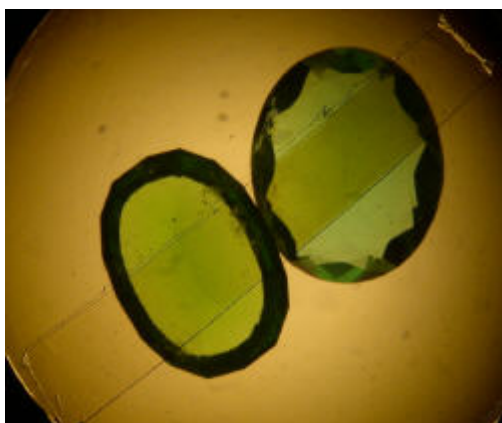
Figure 4.6 Use of an improvised dichroscope to distinguish between immersed gems of green glass (left) and tourmaline (right). The dichroscope was made by attaching a piece of polythene at the 45 degree position to a polarising filter disk, and placing the disk inside the eyepiece of a microscope with the polythene towards the specimen. The plastic strip has to have a retardance of one half wavelength: such a strip can be identified from a number of samples by placing it between parallel polarisers, in which case it appears black, or nearly so. A similar result could be achieved with more difficulty by fitting together three pieces of polarising filter.
