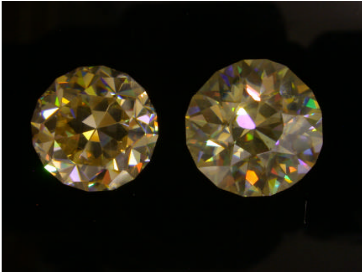
Fig 1.1 Comparison of a non-birefringent gem, strontium titanate, left, with a highly birefringent one, titanium dioxide (rutile) on the right. Although the rutile was cut with the optical axis perpendicular to the table to minimise the effects of birefringence, this property is evident from a few bright facets, which appear double. The rutile and strontium titanate were obtained from Gram Faceting (Jeff Graham) and Osprey Trading (Paul Kessler) respectively.
