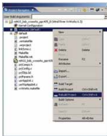
Figure 2 – Workbench build of Xilinx board VxWorks 6 kernel image
