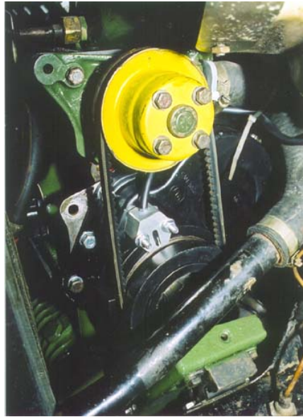
Figure 1 Typical Sensor Fitting on A-Series Engine
