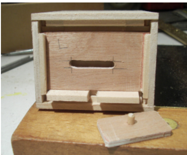
All moving panels have a "holder" panel, which holds that whole panel in place. The holder panel is dropped between the inner box end and the rails. Notice the two pieces of scrap wood holding it at the right height. This holder panel has a slot cut in it for the peg to pass through, and engage in the keyway behind it,
